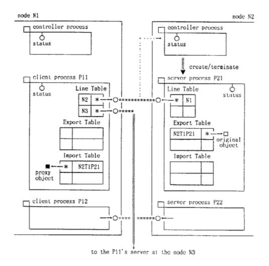
Figure 1: Remote Object Accessing Mechanism (ROAM)
