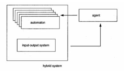
Figure 2: A simple example of a hybrid system with an external agent, in which the role of the external agent is to select an appropriate automaton on the basis of updating variables and evaluating rules and predicates.
