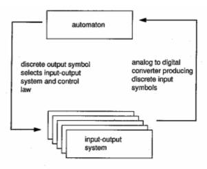
Figure 1: A simple hybrid system in which the discrete digital automaton selects an appropriate inputoutput system and control law.
