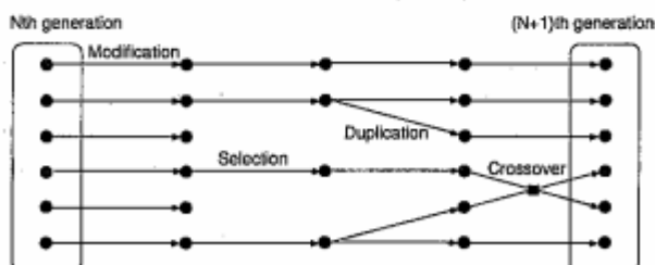
Figure 4: Mechanism of Genetic Algorithm (GA) — GA is a stochastic search algorithms based on the biological evolution process, whose operators consist of modification, selection, duplication, and crossover.
