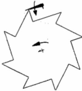
Figure 6: In this state, pushing down on the lever pushes the wheel in a clockwise direction.
