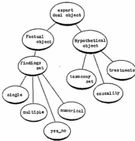
Figure 4. Objects used in the Diagnostic System
