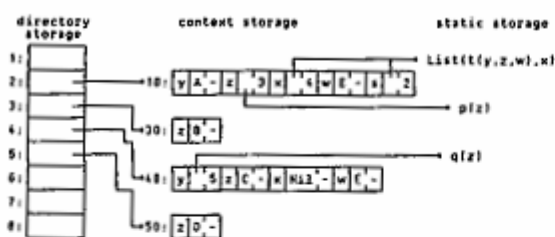
Figure 7. The storage representation of a possible solution to \text{bagof}(s, t(y, z, w), P(y, z)) : s = \text{List}(t(A, p(B), E), \text{List}(t(q(D), C, E), \text{Nil})) . We have assumed that P(y, z) have two solutions, and that w is a non-local variable. The offsets in the directory and the addresses in the context storage are chosen arbitrarily.
